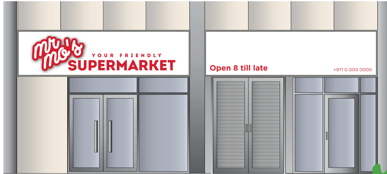
Correct – signage sits between the columns and fits within the designated/recessed
