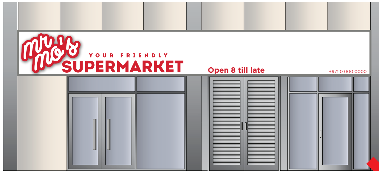
Incorrect – signage should not interfere with the existing architecture and by running across the columns.
